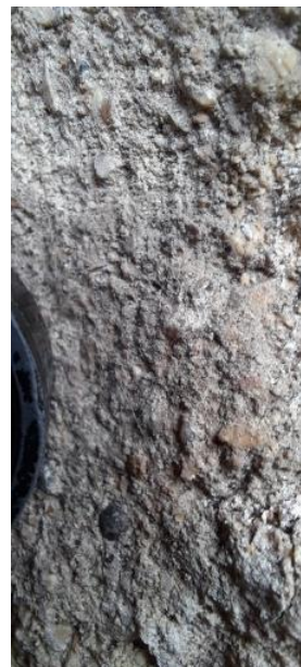
Figure 5: © Roman cement with inclusions.
