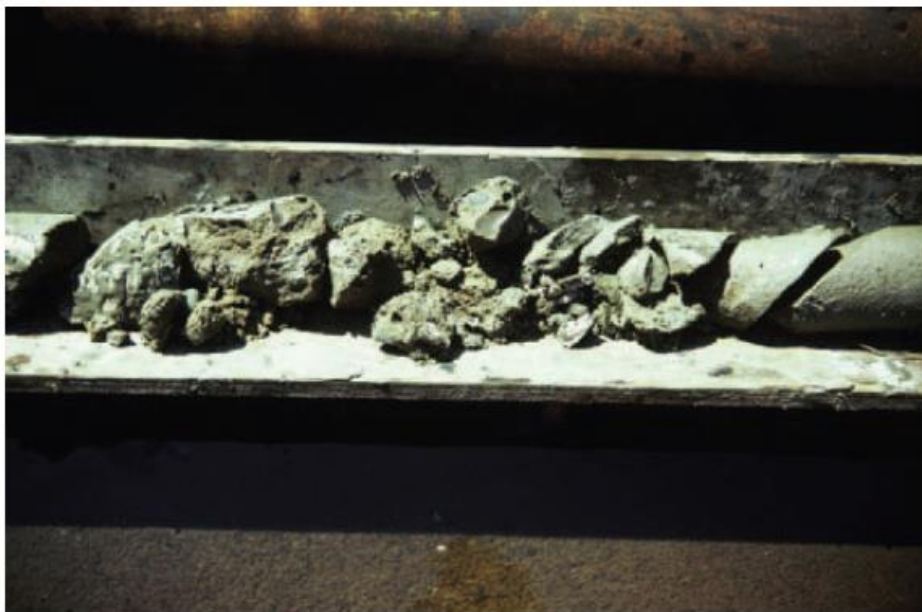
Fig.5. Core of Forties Formation reservoir taken from c.2755-2765m depth in well Forties Delta 52 on 17 May 1982, as part of a programme to assess the feasibility of enhanced oil recovery using surfactants.
